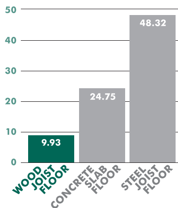
CONSUMPTION OF FOSSIL FUELS (MJ/FT 2 ) ASSOCIATED WITH THREE FLOOR DESIGNS
